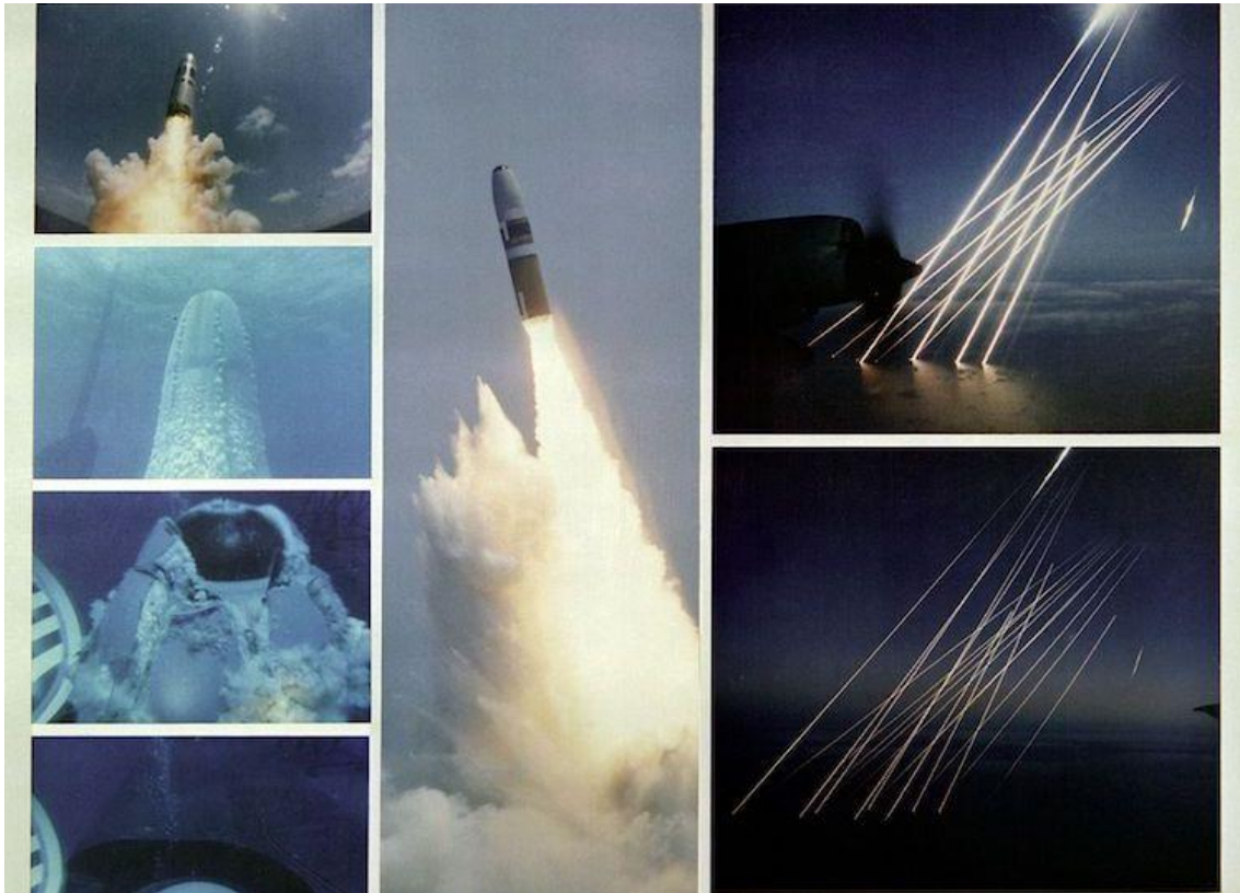
Montage of an inert test of a United States Trident SLBM (submarine launched ballistic missile), from submerged to the terminal, or re-entry phase, of the multiple independently targetable reentry vehicles. 資料：Wikimedia Commons.
