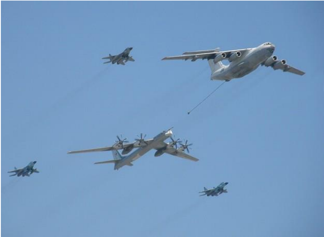
The Tupolev Tu-95 is a large, four-engine turboprop powered strategic bomber and missile platform. First flown in 1952, the Tu-95 was put into service by the former Soviet Union in 1956 and is
