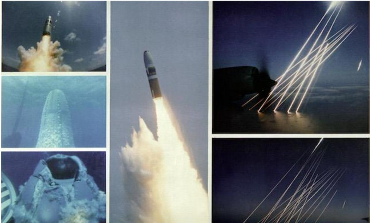
Montage of an inert test of a United States Trident SLBM (submarine launched ballistic missile), from submerged to the terminal, or re-entry phase, of the multiple independently targetable reentry vehicles.
