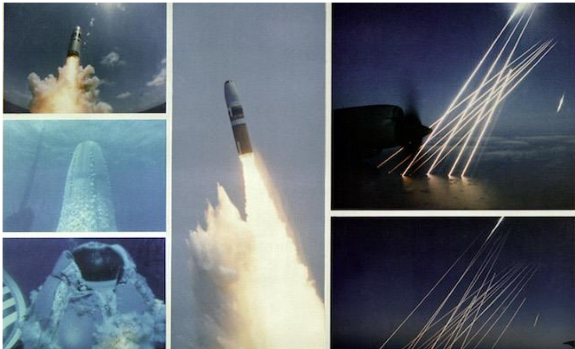
Montage of an inert test of a United States Trident SLBM (submarine launched ballistic missile), from submerged to the terminal, or re-entry phase, of the multiple independently targetable reentry vehicles. 資料：Wikimedia Commons.
